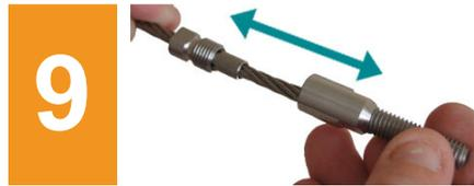
Take the stainless steel body and push onto the cable, eventually bringing the three component parts together. Turn in opposite directions to thread them together.
