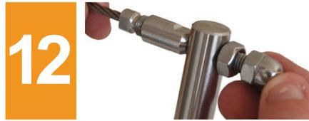
Attach the stainless steel nut and dome nut, Using two wrenches tighten the nuts against each other to create a secure rigid fix.
