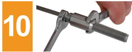
Using a pair of wrenches screw the two sections together until tight.
