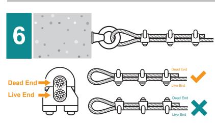
Using 3 wire rope grips - secure the wire cable to create a fixed loop.
